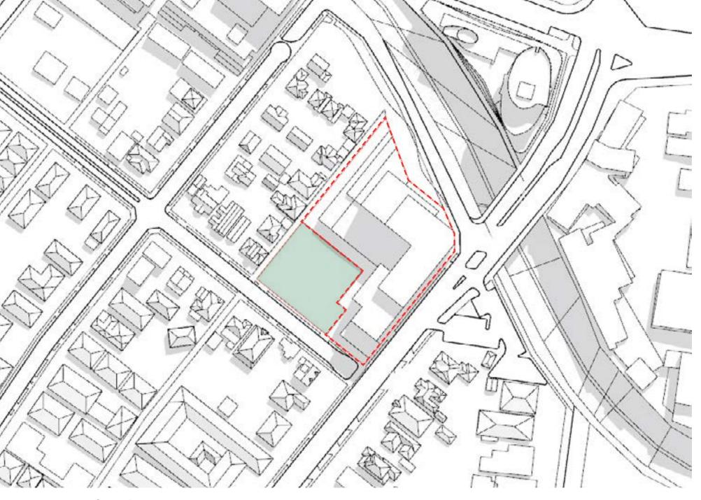
Figure 30. Proposed Shadow Diagrams (22 September)
