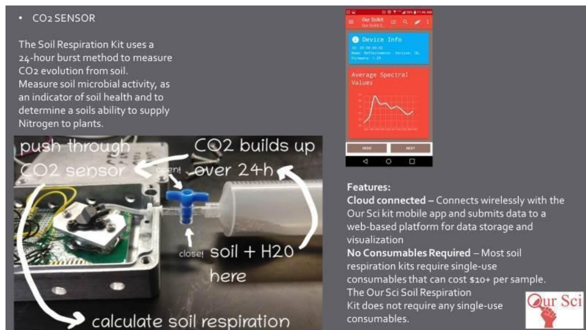
Figure C 3 The Our Sci Carbon Mineralization Sensor (left) connects to an Android-based app (right)
