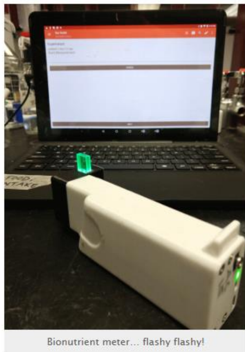
Figure C 5 OurSci – Reflectance Sensor that can be used to measure spectrum on various types of samples liquid and solid.
