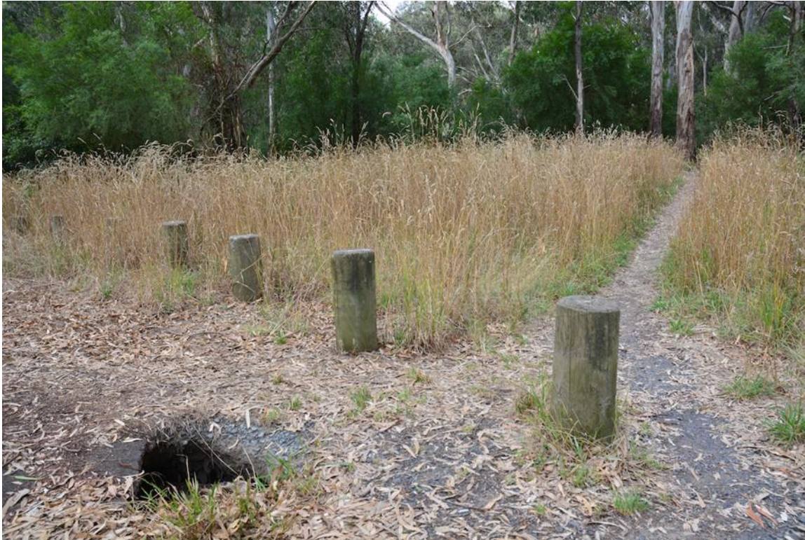
Figure 28 Tunnel erosion identified at the Site.
