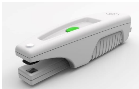
Figure C 2 PhotosynQ - MultispeQ spectrometer
