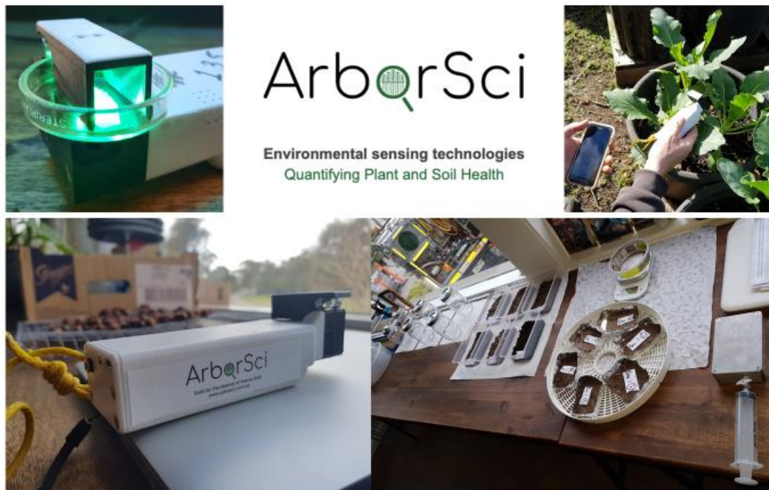
Figure 3 – ArborSci – Reflectometer and Co2 Respiration Chamber Burst Method. Measuring Photosynthesis and Soil Health indicators.
